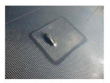
In order to move the triangular ends of the ailerons, you can bend a piece of steel wire (1mm) and glue it into the end of the aileron as shown. Let the wire jut out about 6mm.
