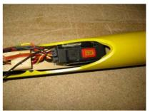
If you want an easy handling of the ready arranged glider, we recommend to mount the switch and the sockets for loading and scanning on a small board as shown.
