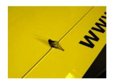
To connect the servos to the levers use two connectors M2,5mm. In between, use a slightly bended welding rod (diameter 2mm), which you solder to the both connectors.
