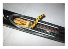
The receiver should be situated close to the opening in the fuselage. In this way, you can change the frequency easily.
